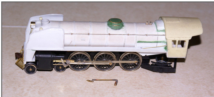
Early shot of 621 (with 624's mechanism) during the valve gear fabrication process
