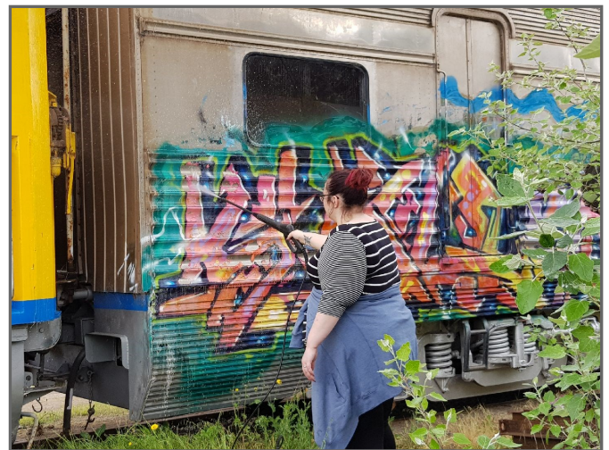
Sherree Cleaning - Sherree hard at work using a high pressure cleaner on the IP Dining Car. The graffiti was three layers thick in some cases and dislodging all of it even with removal fluid was impossible.
