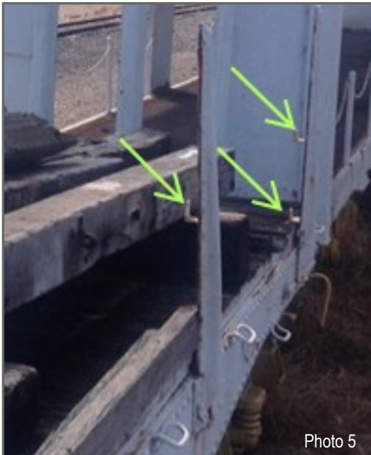
Stanchion bracket detail. Tailern Bend. 01.01.2017. Author photo.
