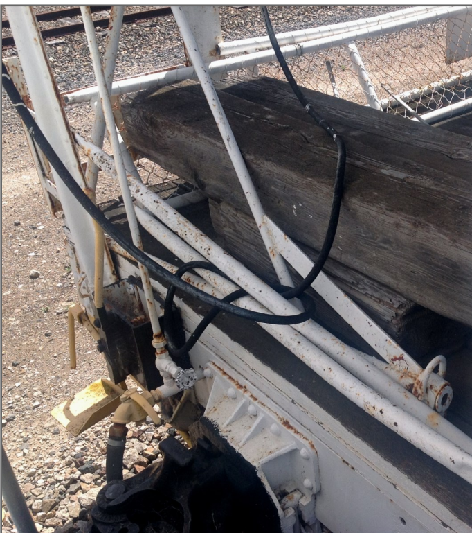
Photo 33 plus detail on next page. Compressed air pipe to crane connection at brake pipe. 01.01.2017 Taillem Bend. Author photo.
