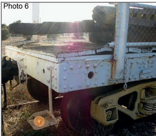
Photo 6 'A' end detail. Shunter's step, condition of deck, dates above bogie. 13.3.2015. Taillem Bend. Norm Bray Photo.
